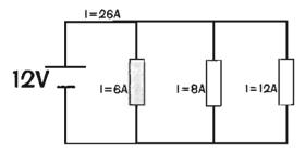
12A in 2 Ohms; 8A in 3 Ohms; 6A in 4 Ohms; 26A in cell.
