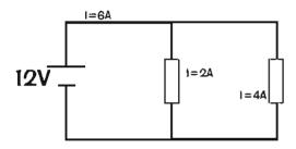
2A in 6 Ohms; 4A in 3 Ohms; 6A
