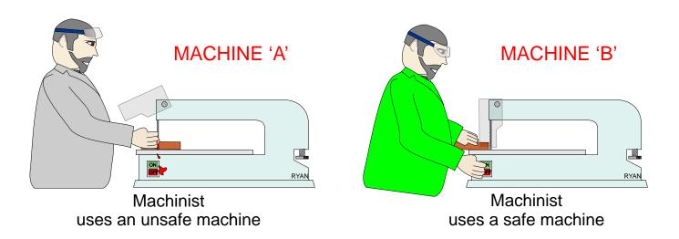
The diagram below shows the micro-switch has been switched on as the guard is in the right position. Also, the 'ON' switch has been pressed simultaneously. This means that the logic states of both inputs are 1 (true, on, high, up).
